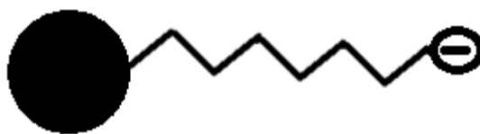
Figure 4-5- A particle (black circle) attached to an anionic surfactant in water.
